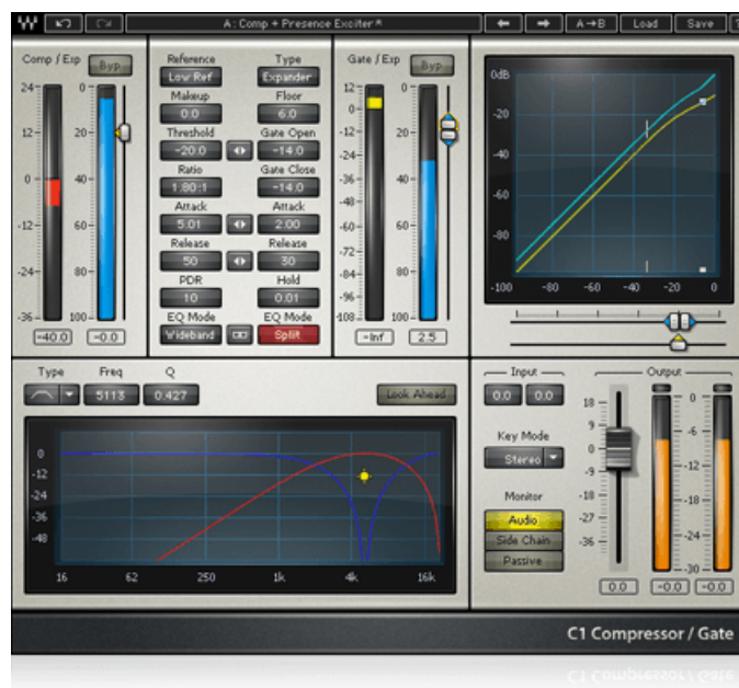
Figure 2.5: Waves C1: The ratio display in the top right gives visual feedback for what would otherwise be an abstract concept. [13]
